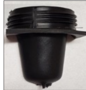
Image 2: Controlled heat focus allows for unique geometries not possible with conventional rotational molding.
