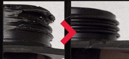
Image 5 & 6: Heat flow could be focused on the appropriate area for improved material dispersion to create improved threading.
